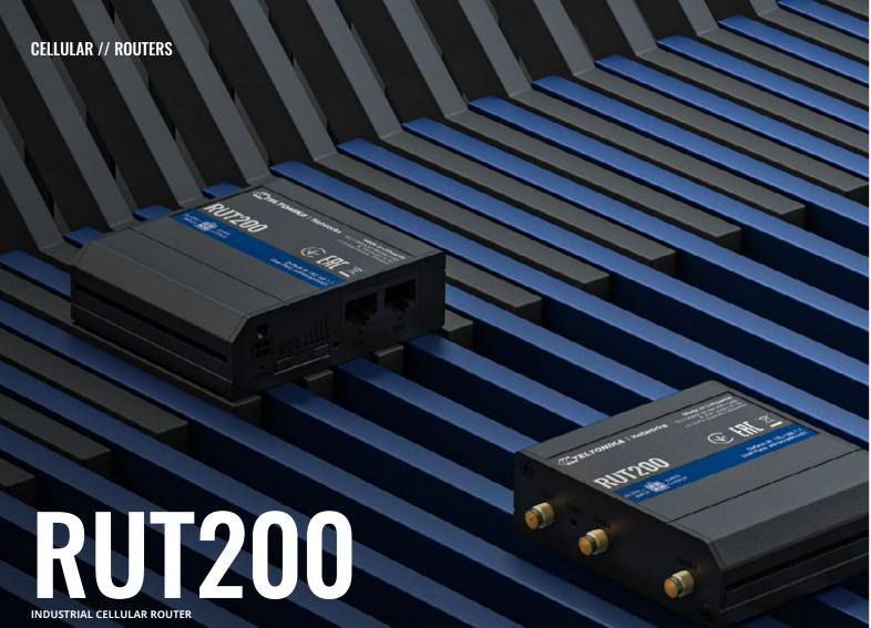
RUT200 is a compact-sized industrial cellular router compatible with the Middle East, Asia, Africa, South America, and CIS networks. Featuring multiple connectivity options (LTE, Wi-Fi, and Ethernet), this model is perfect for quickly setting up primary and backup connectivity with remote management capabilities.
