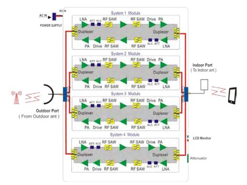
Quadruple band booster Diagram
