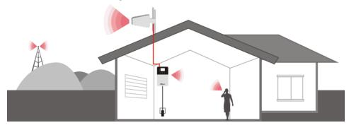
1-Outdoor directional antenna 3-Booster with built-in indoor antenna
